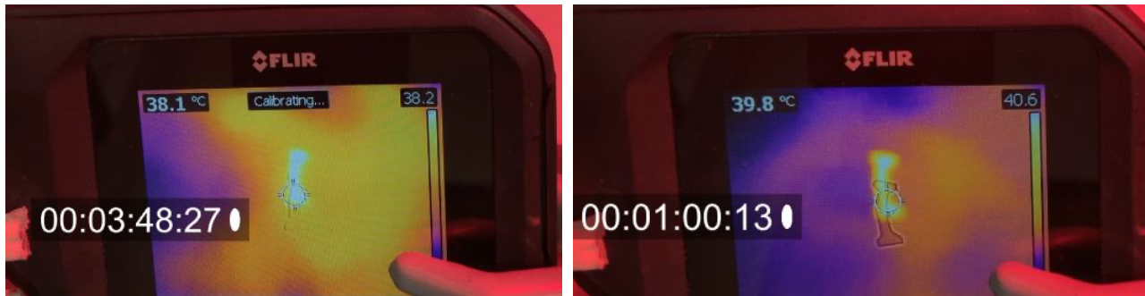
Figure 6: TNI test setup, with plain sample (left) reaching TNI in a shorter time than the CNT (right) sample
